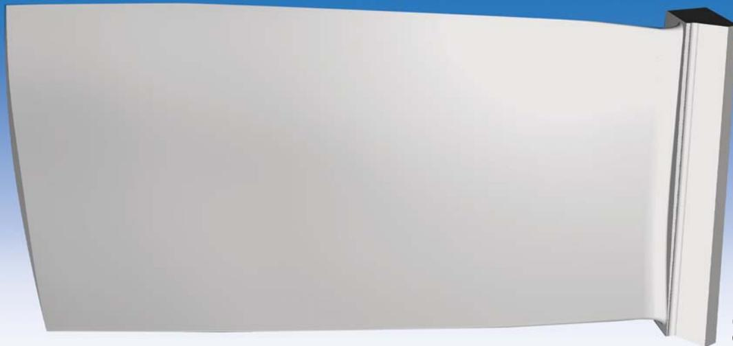
CAD model of redesigned compressor blade
