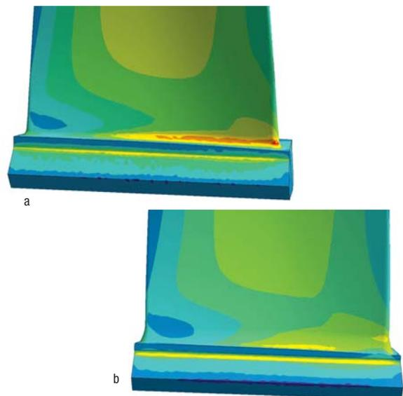
Closeup of the maximum principal stress on the pressure side of (a) the original equipment manufacturer's blade and (b) the redesigned blade
