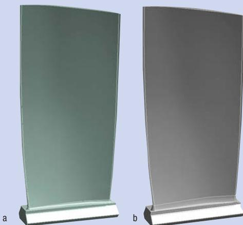
Geometry of original equipment design (a) and modified geometry (b), as created using ANSYS DesignXplorer software
