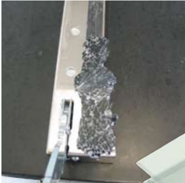
Glass on a prototype oven door broke due to high thermal loads.
