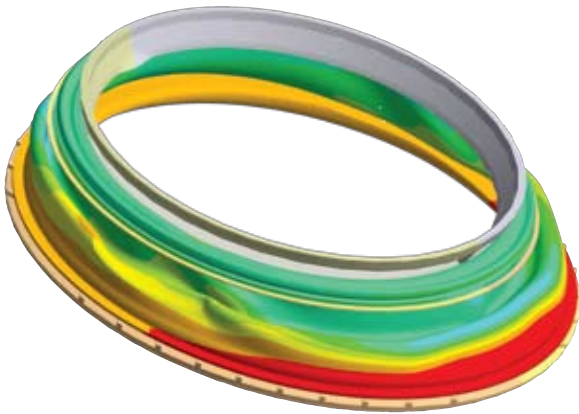
The rubber bellow was completely meshed with four-noded tetrahedron elements, which saved considerable time.
