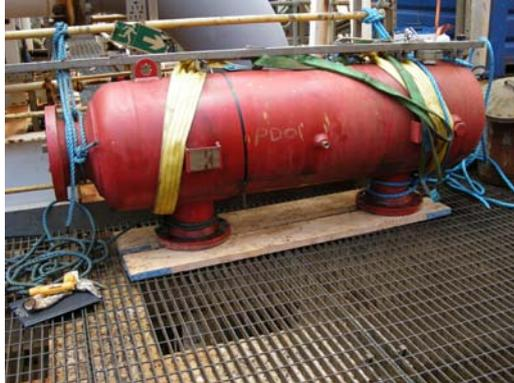
Gas dampers draw gas or oil from the seabed and transport it to a storage tank. Upstream of the gas damper a scrubber extracts moisture from the flow. On entering the gas damper assembly, the flow velocity of the gas or oil is reduced, and any remaining water/moisture content that might have slipped through is removed. Downstream, the gas is compressed and sent off to storage ready for transportation.
