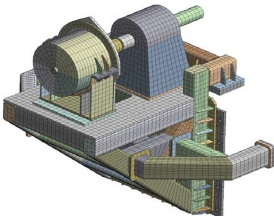
This case study describes the design and analysis of a support structure for a braking system that was used for a huge flywheel generator. The flywheel generator was designed as a motor generator unit used by the Max-Planck-Institut für Plasmaphysik (IPP) in Garching, Germany, to provide a considerable amount of power for their experiments. IPP is investigating the physical principles underlying a plasma fusion power plant, to produce energy.
