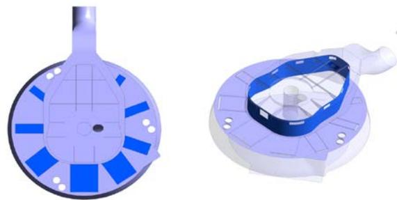
Based on the above results from the original design, the geometry of the slots was modified in order to try and gain a more balanced flow throughout the hood.
