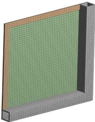
The geometry for this analysis was created within ANSYS and the quarter symmetry Finite Element (FE) model can be seen in the graphic to the left. The blast vent panel was made up of a single skin of steel plate which was spanning on to a supporting steel structure. The model was meshed entirely with membrane elements.
